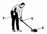
Which of the positions labelled P, Q and R would represent the load, effort and fulcrum when the machine is in use?
