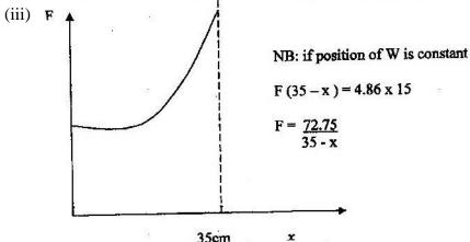
(iv) As x increase/ anticlockwise moments reduces/ moments to the left reduces/ distance between F and pivot reduces F has to increase to maintain equilibrium
